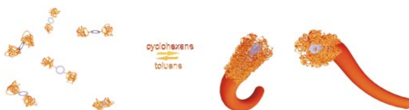
Figure 5. Schematic representation of the aggregation of the block copolymers into hollow cylindrical brushes. The PS block is the corona (orange) and the rigid ring is located in the core (blue) (not in scale).
